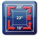
Traditional radiator systems send heat up under the ceiling where it is cooled off and returns along the floor as cool draughts.
