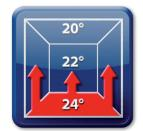
A DEVI floor heating system distributes the heat across the floor surface and leaves the rest to the natural law that heat rises.
